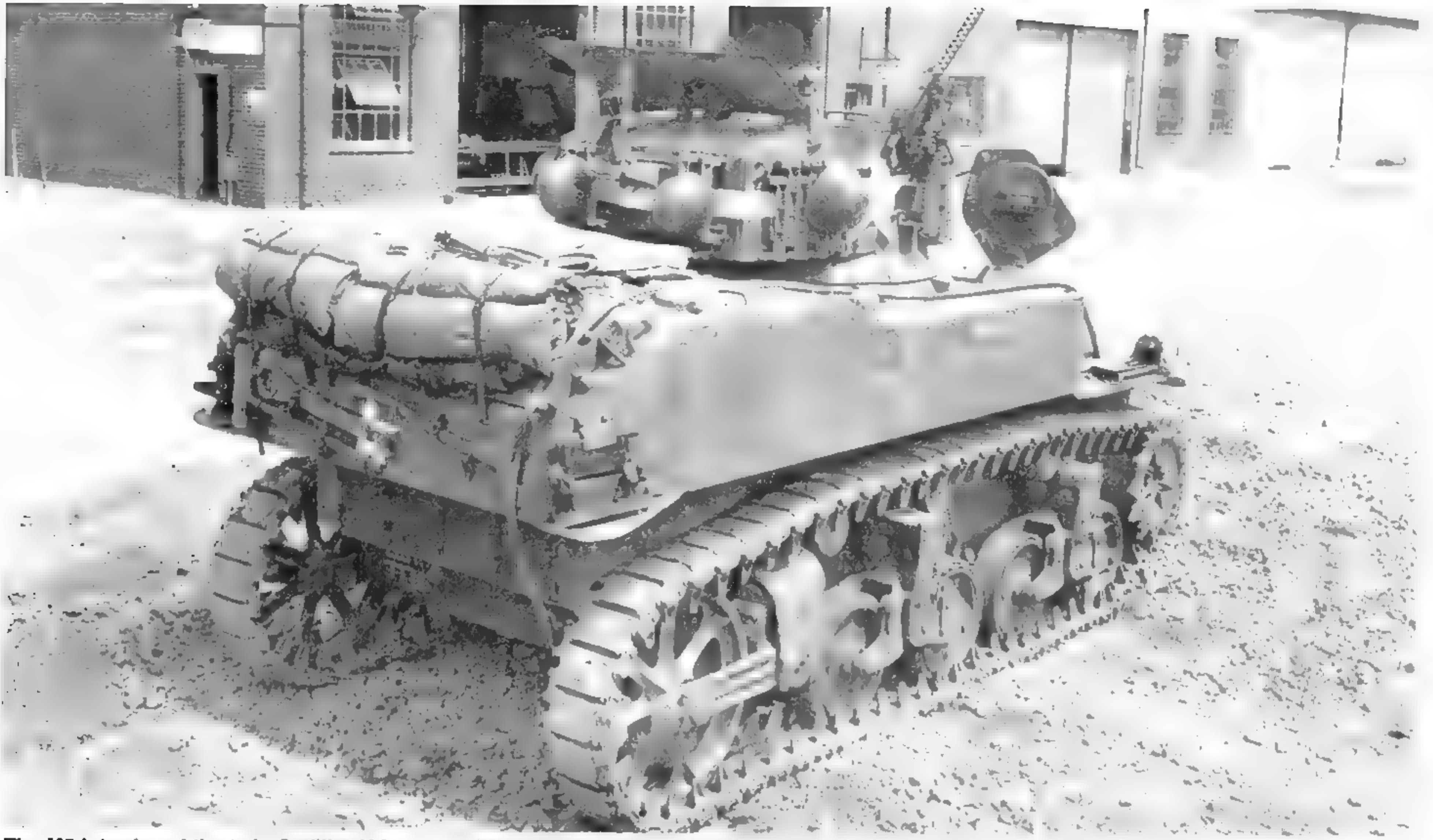
The M5 introduced the twin Cadillac V-8 power plant that was used in many later tanks. (Photo courtesy of the Patton Museum)
